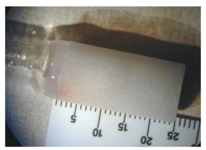
Figure 6. A fine red powder (consistent with red phosphorus) was found to be trapped in the ground glass diffuser of Trap 01 during both cook stages. It is assumed that this came from particulate suspended in the vapors because there was never any liquid transfer from the reaction vessel into the vacuum line. The trapped powder diffused approximately 5mm into the ground glass diffuser indicating a very fine particle size.
