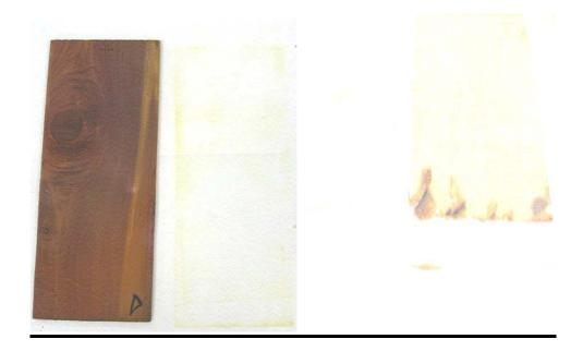
Figure 2. This (left) is the exposed cedar shown next to the residue left against white butcher paper after contact overnight. Wallboard (right) which has been exposed seems to take on the purple iodine color when compared to unexposed wallboard.
