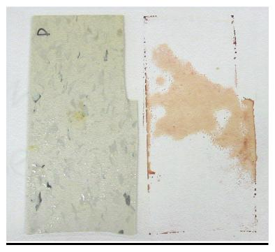
Figure 3. The acidic vapors which condensed onto the linoleum reacted with butcher paper to leave this characteristic red staining. Note the blotches of yellow stain on the linoleum.
