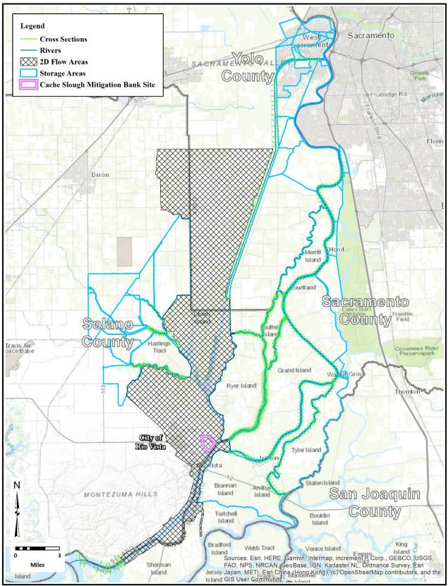
Figure 7. Tidal Hydraulic Model Schematic
