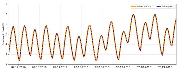
Figure 19. With- and Without-Project Tidal Stage Hydrograph, Cache Slough at Steamboat Slough, Winter Season
