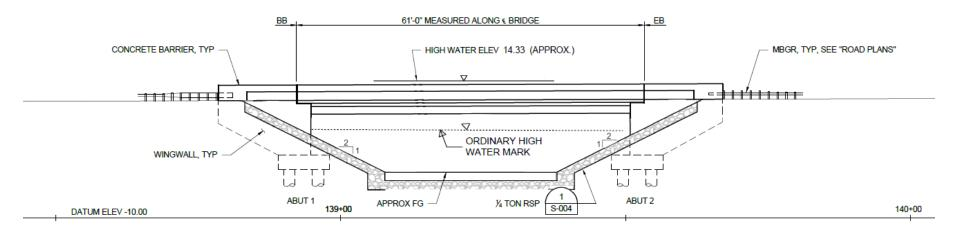
Figure 5. Proposed State Route 84 Water Control Structure
