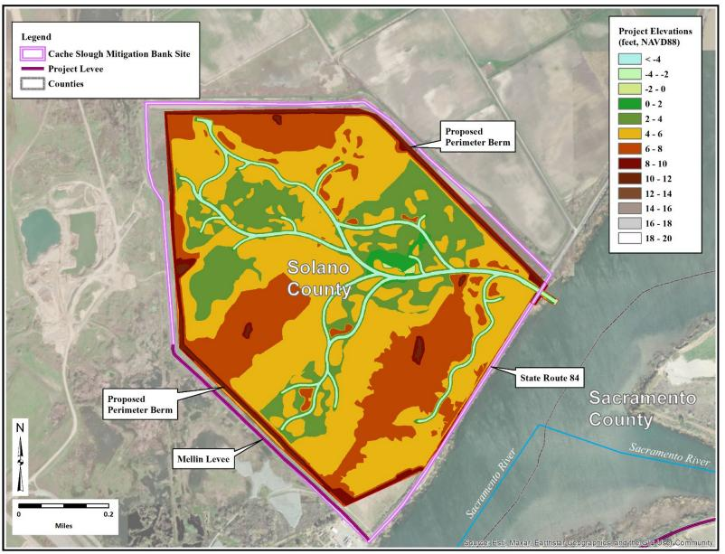
Figure 4. Restoration Plan - Grading
