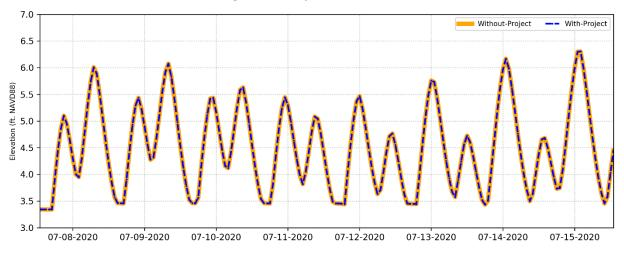
Figure 28. With- and Without-Project Tidal Stage Hydrograph, Lookout Slough Tidal Habitat Restoration and Flood Improvement Project, Agriculture Operation Season
