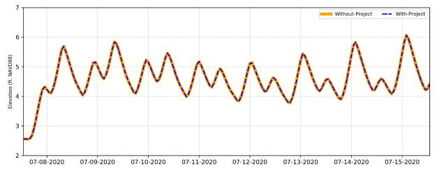
Figure 26. With- and Without-Project Tidal Stage Hydrograph, Prospect Island Tidal Habitat Restoration Project, Agriculture Operation Season
