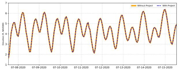
Figure 25. With- and Without-Project Tidal Stage Hydrograph, Cache Slough at Steamboat Slough, Agriculture Operation Season
