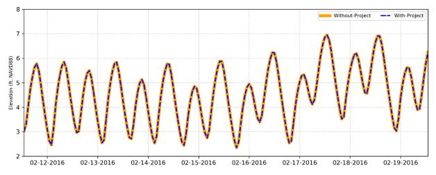
Figure 21. With- and Without-Project Tidal Stage Hydrograph, Lindsey Slough at Yolo Bypass, Winter Season
