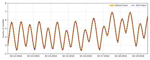
Figure 18. With- and Without-Project Tidal Stage Hydrograph, Watson Hollow Slough Siphon, Winter Season
