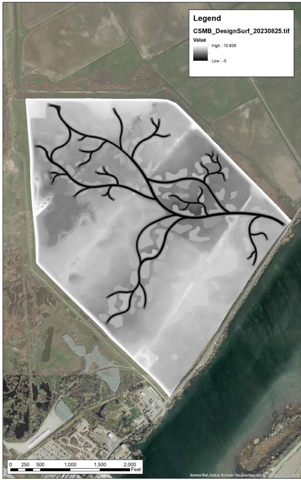
Figure 10 CSMB restoration design.
