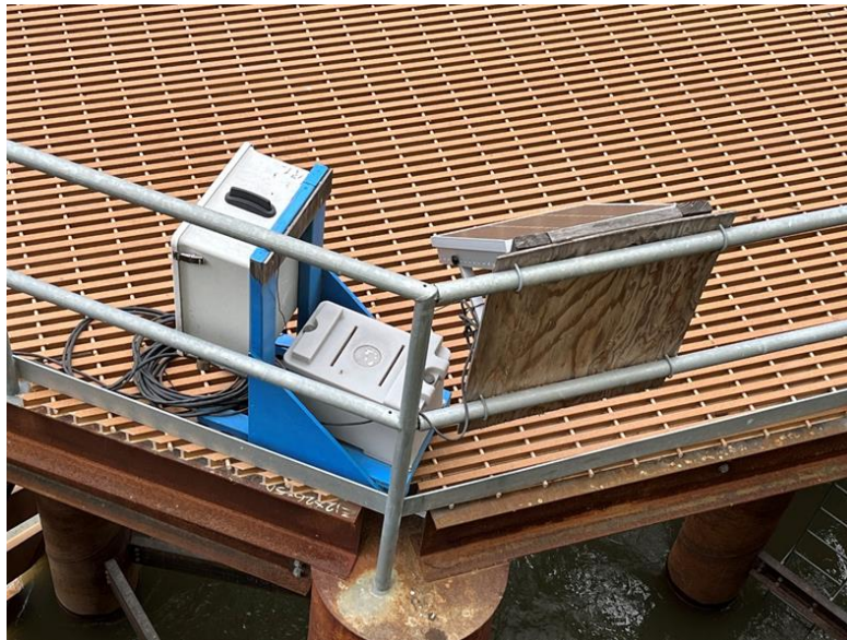
Figure 3. Example of a real-time land based sturgeon telemetry station with communication boxes and solar panel. Acoustic sensors are fixed at the bottom of the water body and connected to the station with a long cable.
