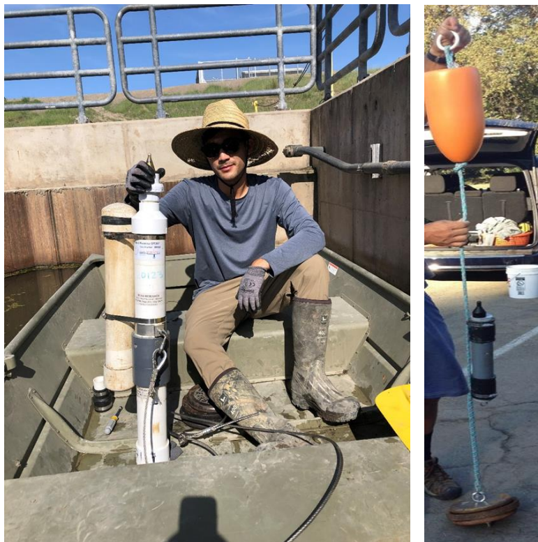
Figure 4. Examples of autonomous telemetry receivers with anchors and different types of flotation devices (Left - receiver attached to floating tube. Right – receiver in between float and anchor).
