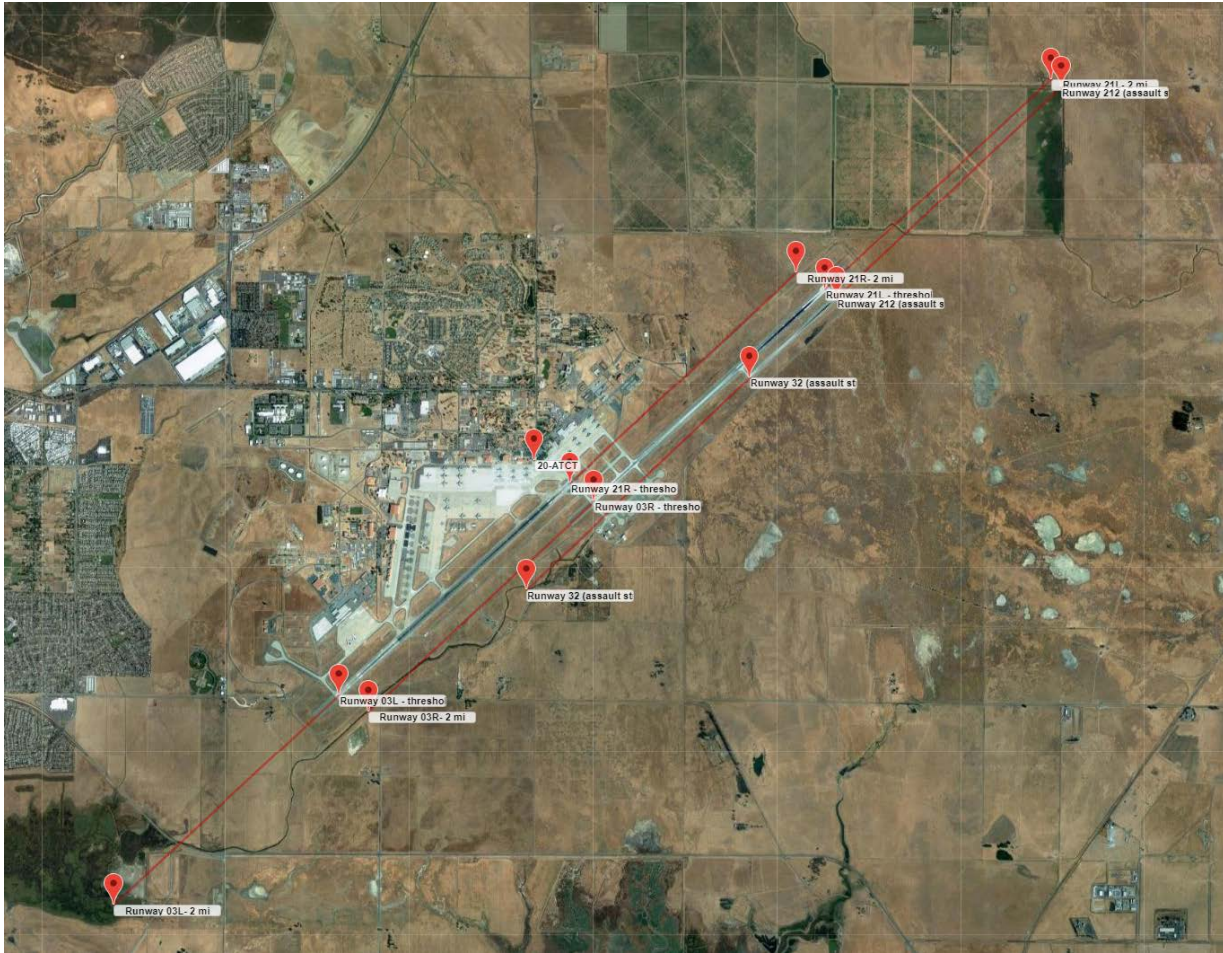
Figure 5. Approach Flight Paths (Red Lines) to Travis Air Force Base’s Six Runways and the Airports Air Traffic Control Tower (“20 – ATCT” slightly to the left of the center of the image), as Modeled in ForgeSolar
