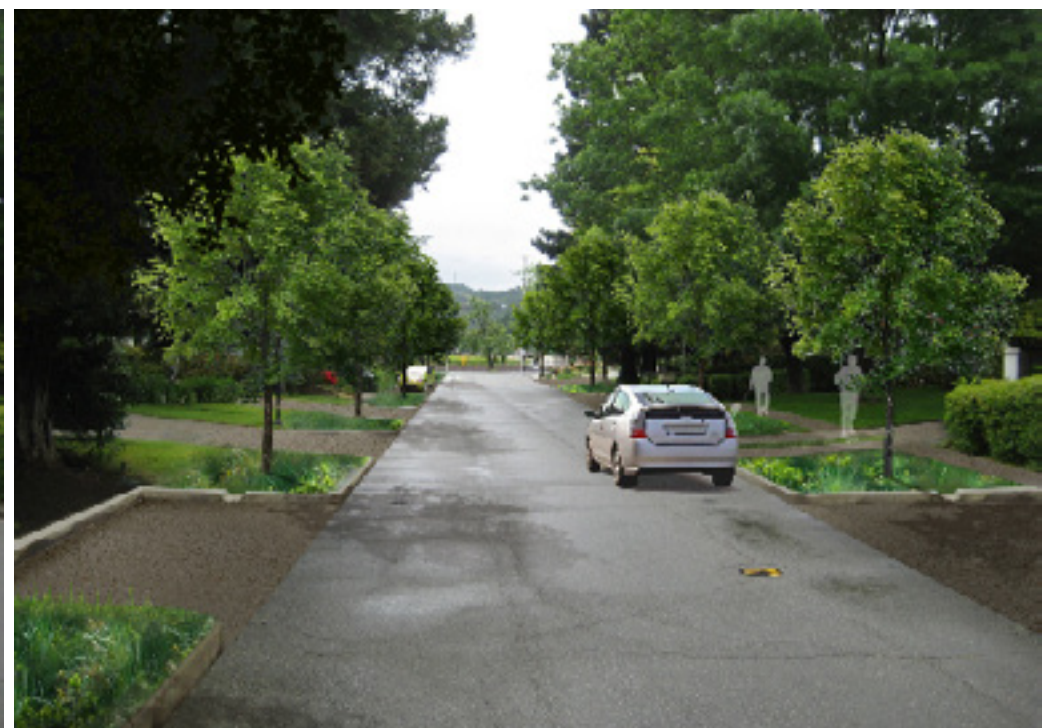
Figure 3-14: Roads and Streets Sustainable Design Approach - By utilizing a more efficient site design, the space can be used for stormwater infiltration and additional landscaping to encourage slower vehicle speeds and increase pedestrian safety.
