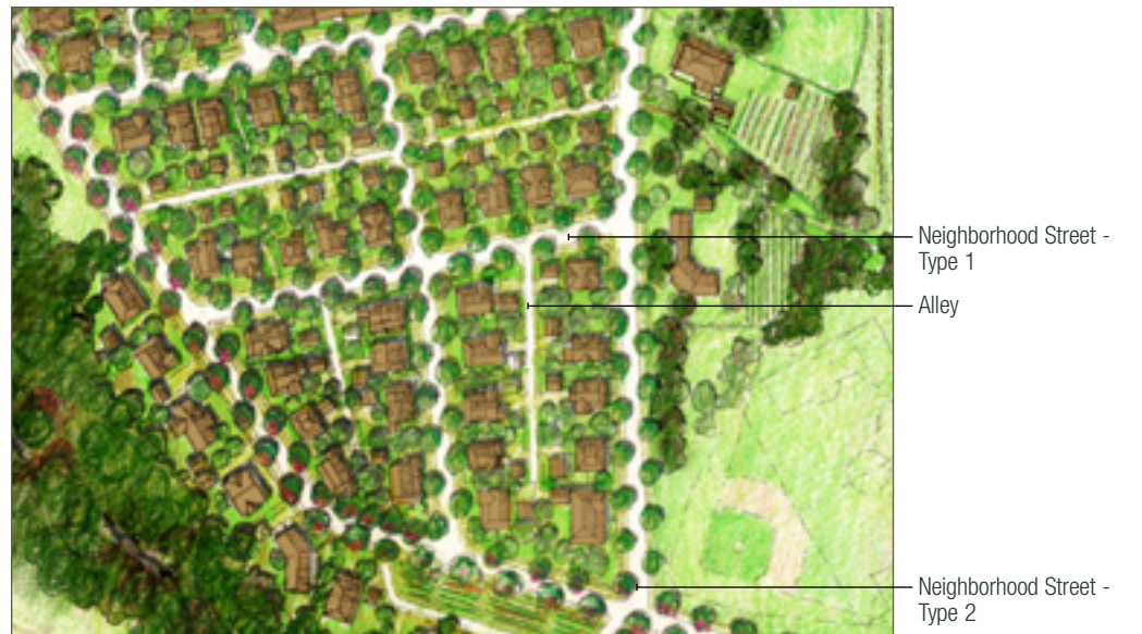
Figure 3-25: Elkhorn Street Network Detail
