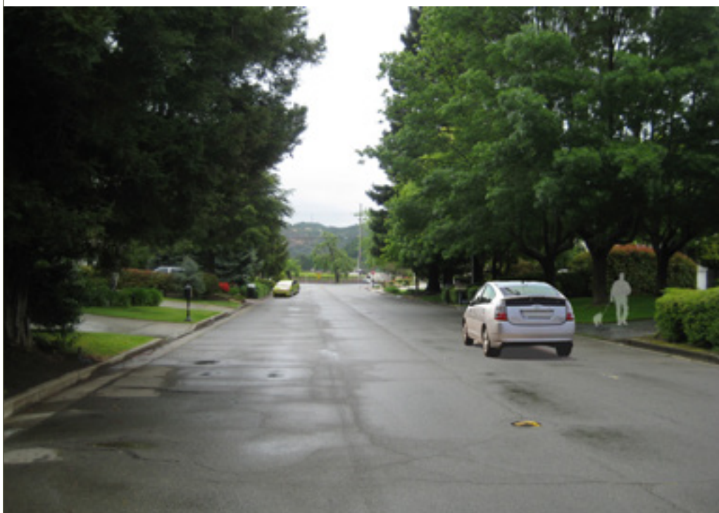
Figure 3-13: Roads and Streets Typical Design Approach - This suburban street is almost 100% impervious and designed primarily for auto flow. This combination contributes to higher auto speeds and large quantities of stormwater runoff.
