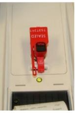
□ Plug the Ballot Scanner power cord into a wall outlet. A green light will illuminate on the power brick when AC power is present.
