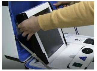
Verify that the vDrive cover is sealed with number on security log. This seal will not be removed. If it does not match, notify the Inspector who will contact the Registrar of Voters Office at 707-784-3375.
