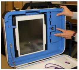
Plug power cord into brick, then plug power connector into back of Ballot Scanner, flat side up.
