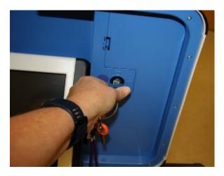
□ Unplug the Touch Writer from AC power. Separate the power cord from the power brick.
