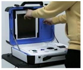
□ Proceed to seat the tablet firmly in the cradle, tilt back and lock into place.
