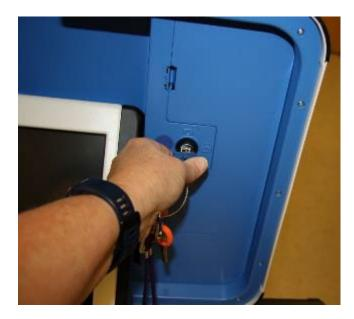
□ Make sure vDrive compartment of Ballot Scanner is sealed with number on the Security Log.
