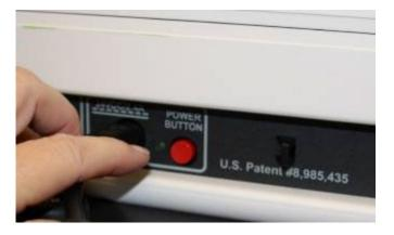
□ When the Ballot Scanner is completely powered down and is displaying a black screen, unlock the tablet using the blue key.
