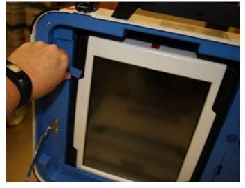
$\hfill\square$  Lock the tablet in place with the blue key.
