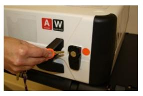
□ Open the storage compartment and remove power brick and cord (this does not require a key).
