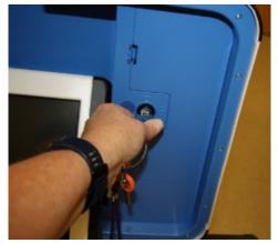
□ Using two hands, gently remove the tablet from the cradle and stow in the storage area in the case cover. Move the latch to hold the tablet in place.
