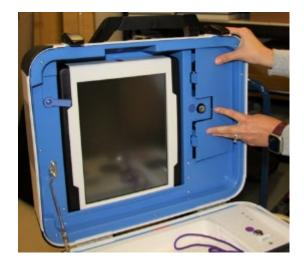
□ Unplug the laser printer from the back of the Touch Writer.
