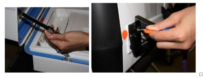
□ To remove Ballot Scanner from Ballot Box, reach inside Ballot Box and pull cord toward you. This will unlock the Ballot Scanner from the Ballot Box.
