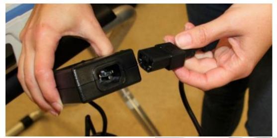
Unplug the power cord from the back of the Ballot Scanner. The power cord has a locking connector. To disconnect the power cord, grasp the cord at the base of the black connector molding and slide back the sleeve. This will unlock the connection so that the cord can be removed.
