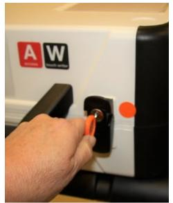
□ Reaching under the Touch Writer table, pull the metal latch toward you to unlock the Touch Writer from the booth.
