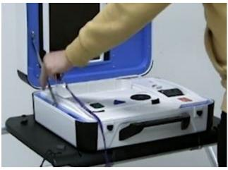
□ Use the blue key to unlock, unlatch and remove the tablet from its position.
