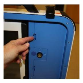
Remove power brick and cord from storage compartment and from the Ballot Scanner case, replace storage compartment cover, then close lid of scanner.
