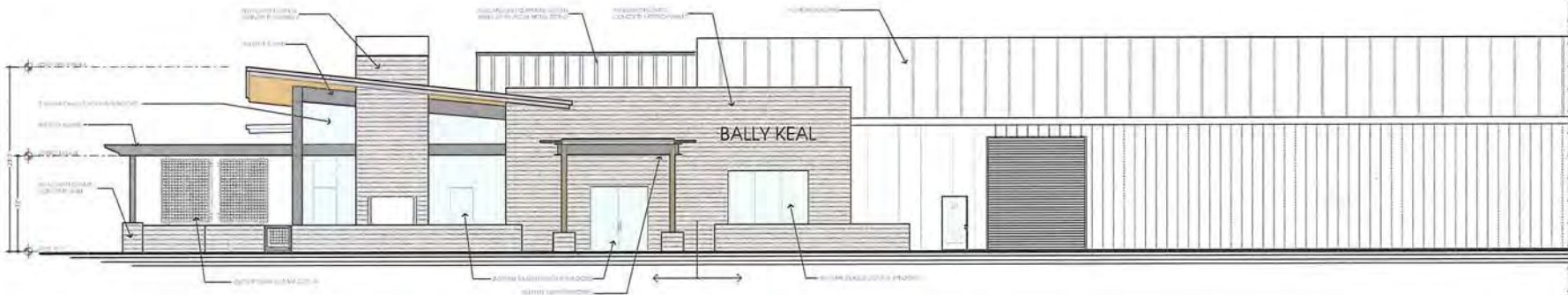
2 TASTING ROOM NORTH EXTERIOR ELEVATION A-2.2
