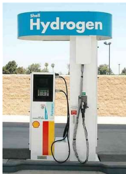
Hydrogen Fulling Station
