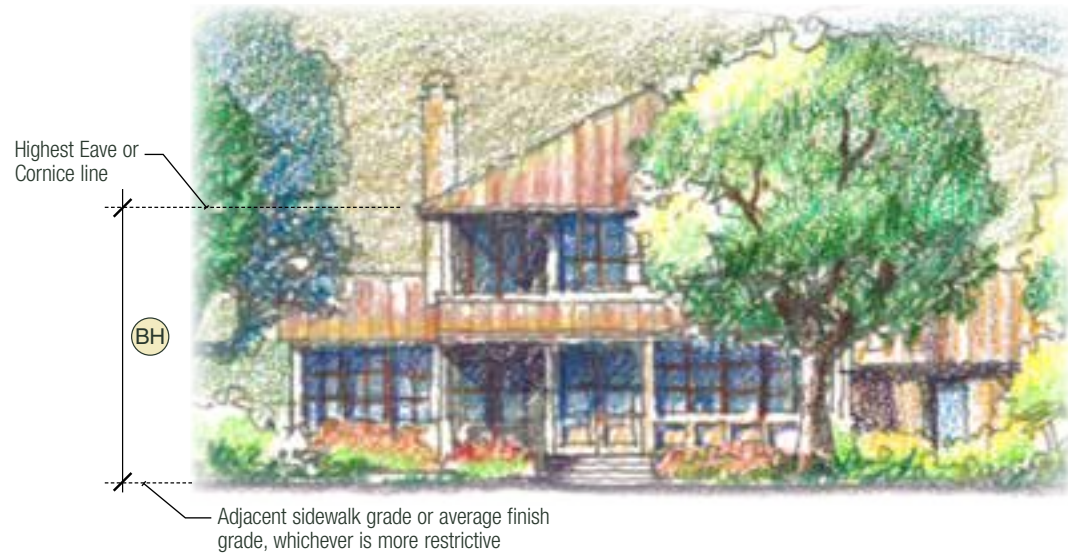
Figure 5-41: Building Height Diagram on gently sloping site
