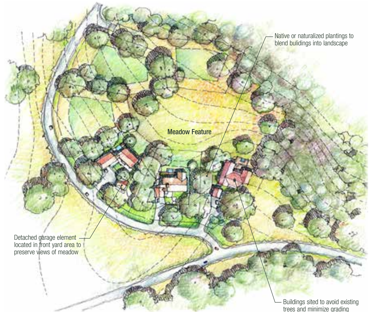
Figure 5-29: Meadow: Conceptual Site Plan - Buildings located at the edge of meadow clearings
