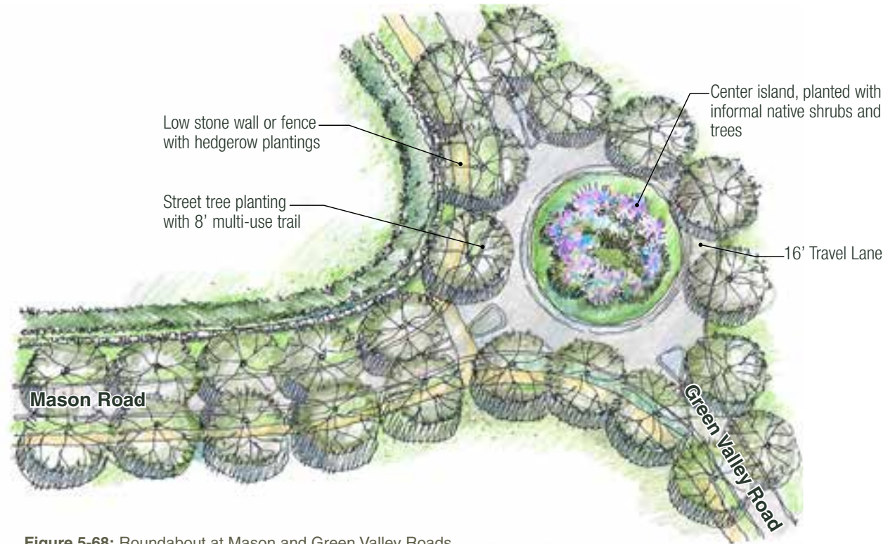
Figure 5-68: Roundabout at Mason and Green Valley Roads
