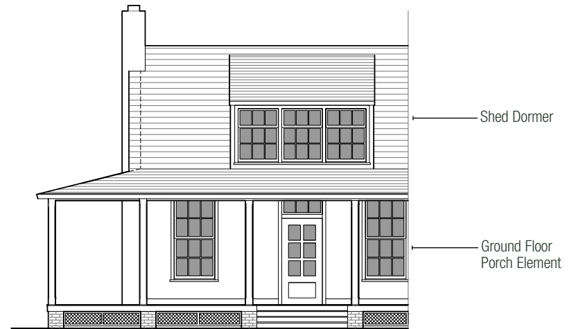
Figure 5-26: Farmstead Frontage Design - Wrap-around Porch
