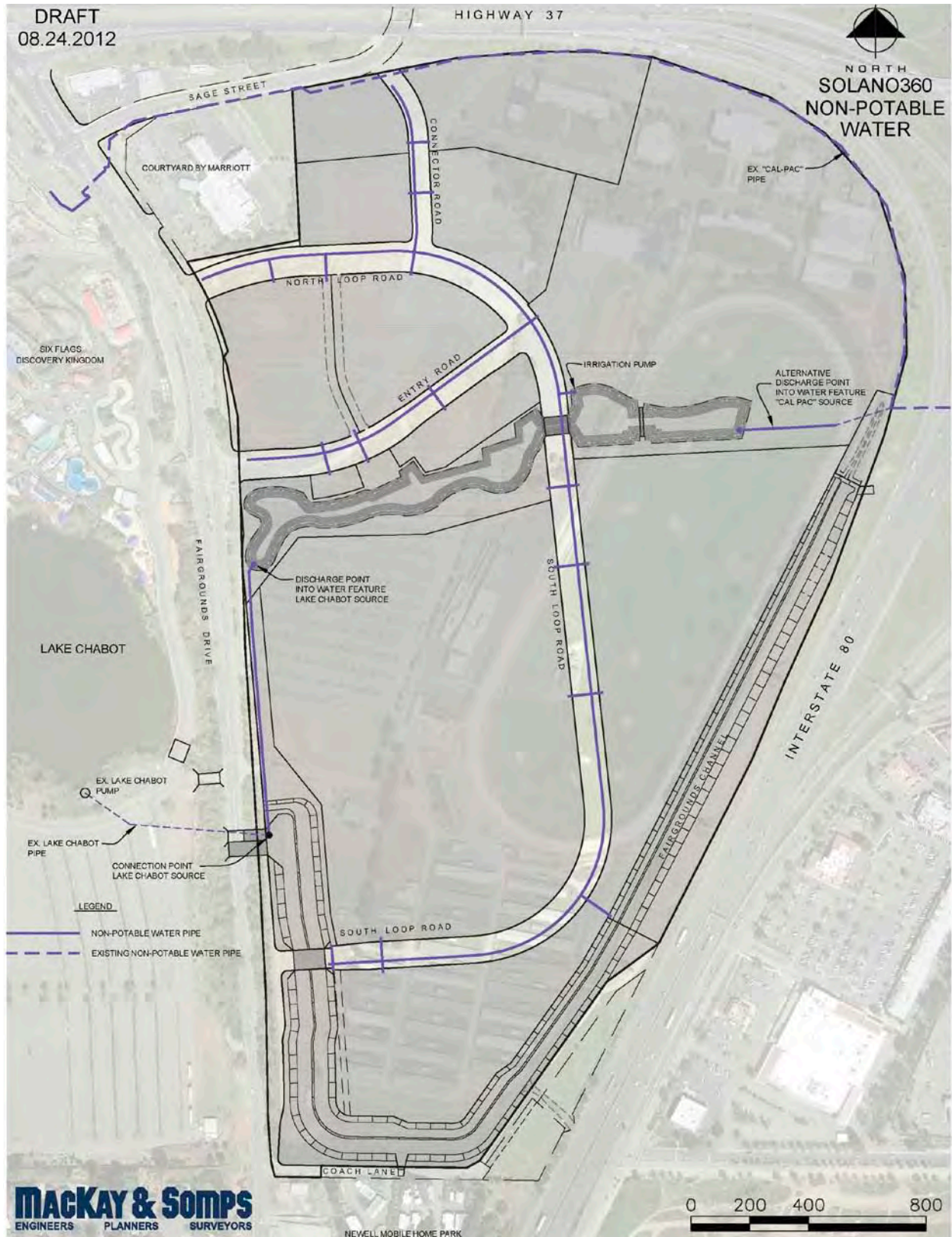
Figure 6.3: Non-Potable Water Exhibit
