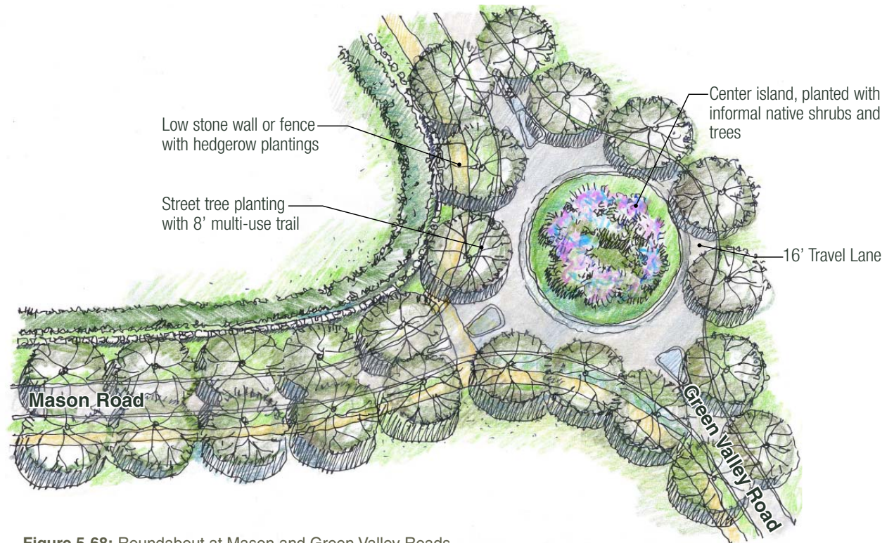
Figure 5-68: Roundabout at Mason and Green Valley Roads
