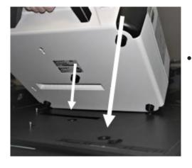
Remove the Ballot Scanner from the equipment caddy and place it on the Ballot Box. Place feet on bottom of the Ballot Scanner into indentations on top of the Ballot Box.
