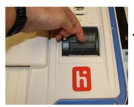
Pull up the small piece of plastic over the printer.
