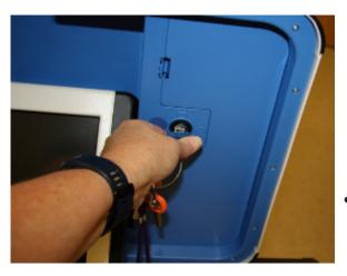
• Lock the tablet in place with the blue key.
