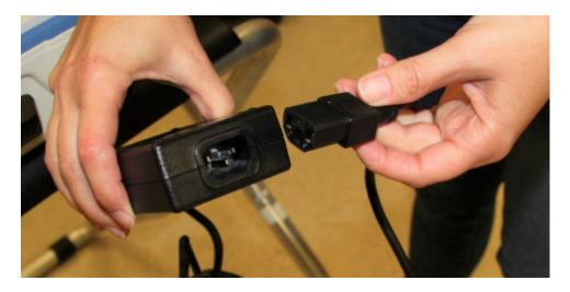
• Unplug the power cord from the back of the Touch Writer. Note that there is a locking sleeve that must be pulled back from plug on back of Touch Writer! To disconnect the power cord, grasp the cord at the base of the black connector molding and slide back the sleeve. This will unlock the connection so that the cord can be removed.
