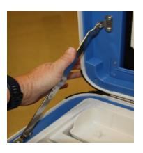
• Unlock (blue key), unlatch and remove the tablet.
