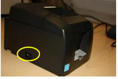
• If your printer is not already on press the switch on the left side of the printer to power it on. The power button light will turn green. (This step is only necessary if the printer is not already on).
