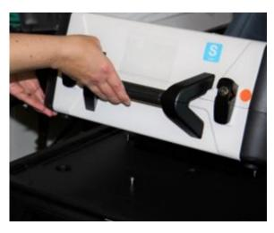
• Grasping the handles, lift the Ballot Scanner up off the Ballot Box and place the Ballot Scanner on the equipment caddy.
