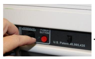
Press the red power button on the back of the Ballot Scanner to power it on.
