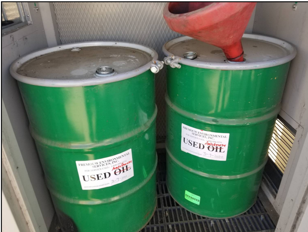
46 : View of two 55-gallon drums of used antifreeze. No signs of leaks or spills were observed.
