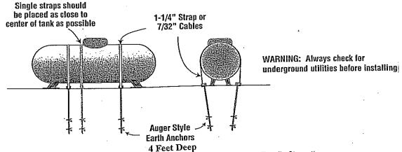
Strap: 1-1/4" X .031 Galvanized Steel, Class B, Grade 1, 4725 Tensile Strength.
