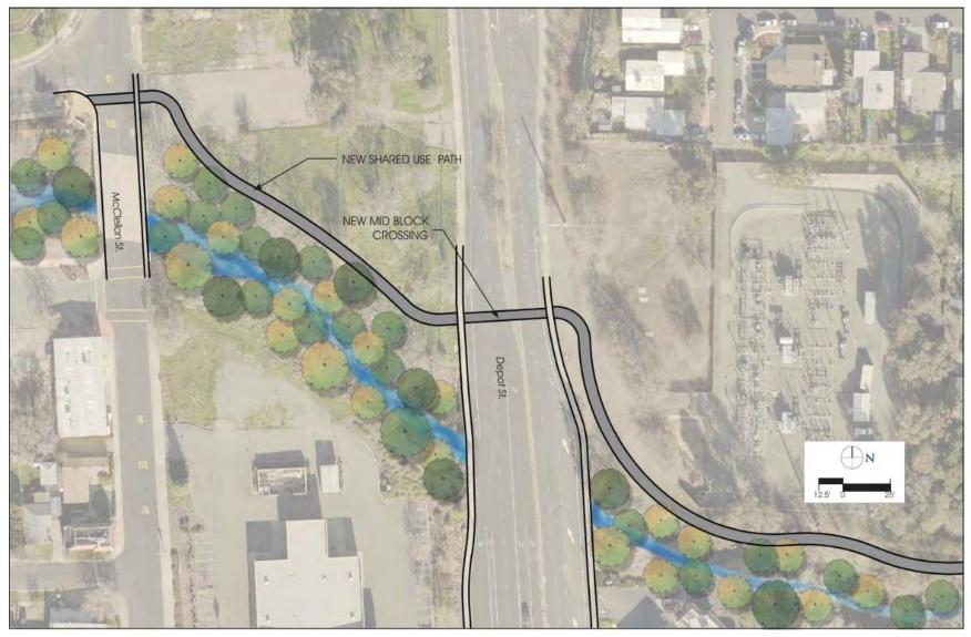
Figure 4.5.2-14: Ulatis Creek Class I Bike / Shared-use Path Illustrations are for conceptual purposes only and further analysis is needed.
