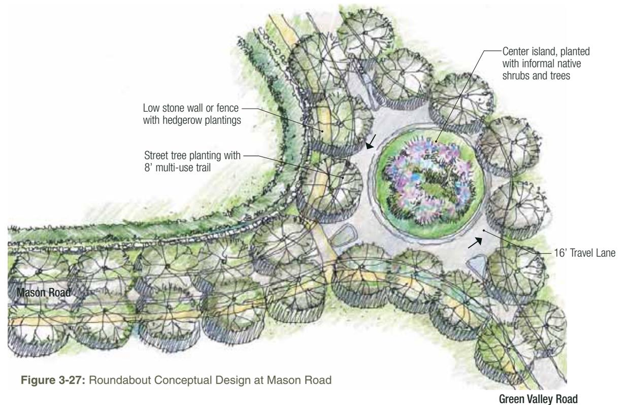
**Figure 3-27:** Roundabout Conceptual Design at Mason Road
