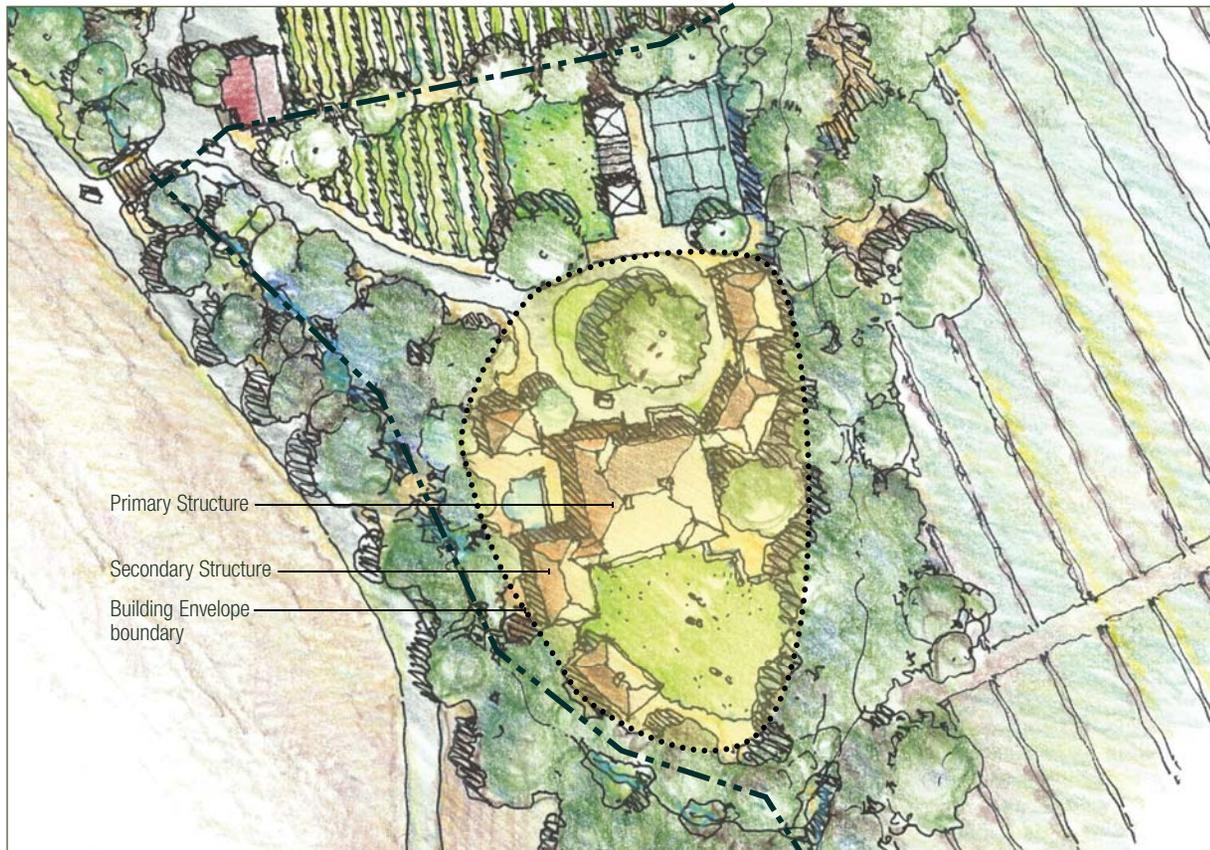
Figure 5-34: Compound Building Envelope Diagram
